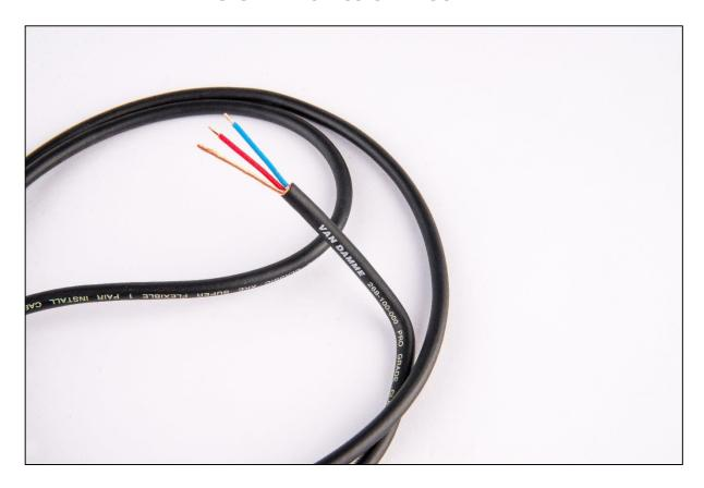
Van Damme Super Flexible 1 pair is a 3.60 mm balanced analogue audio cable with a lapped copper spiral screen. This cable is ideal for use with miniature connectors such as the Switchcraft Tini-Qg range and other small connectors typically found on Lavalier microphones. Its helical spiral shield can withstand multiple flexing operations making it preferable to foil screened 1 pair for certain dynamic applications.
