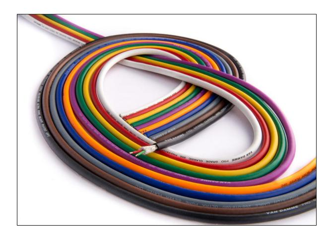
Van Damme Pro Grade Classic XKE Pro-patch cable has been specifically designed as a 4.85mm overall diameter cable to suit Neutrik and Switchcraft bantam jacks, and other applications requiring a lower OD cable. Its braided screen and tightly packed construction ensure that the smaller size in no way compromises the mechanical and sonic integrity.
