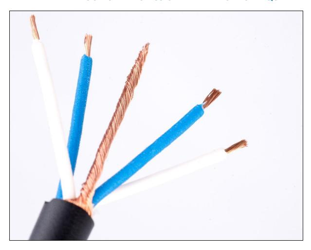
Based on the proven Van Damme 6.00mm Classic Starquad, this miniature version features the same conductors but has a helical lapped copper screen for greater flexibility. Its overall diameter of 4.85mm makes it ideal for bantam adaptor cables, short patchcords and boom microphone cables. The starquad construction ensures excellent rejection of EM and RF interference.
