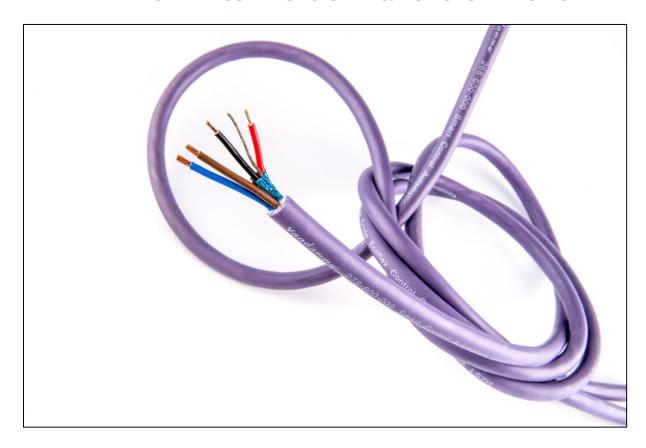
This range comprises a PVC or LSZH jacketed home automation control cable Van Damme Smart Control home automation cables are primarily for use with common automation system control found in home and office environments. These systems run a screened twisted pair with an additional 2 wires for DC voltages used, for example, for powering remote programmable touch panels.
